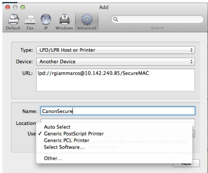
Filter the list to find your device's PPD. In this example we are finding the Canon iR-Adv 400/500 PS.
