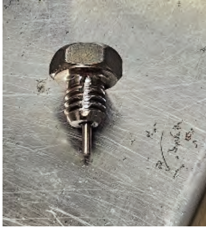
Titanium cranial port for intracranial pressure monitoring in macaques.
