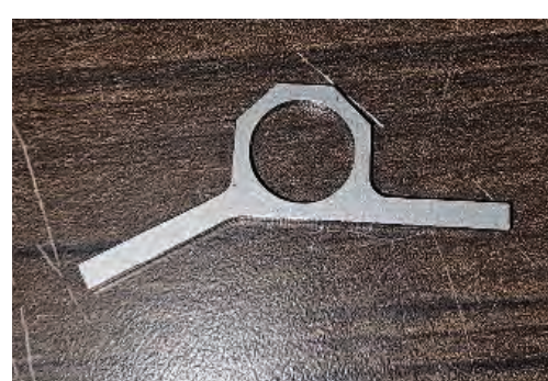
Titanium headframe for fluorescence imaging in mouse cortex.
