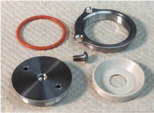
Titanium sub-dermal cranial implant and PEEK cortical window for macaque 2-photon imaging.
